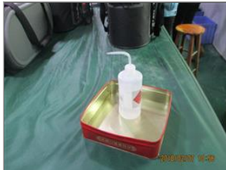
Photo of chemical storage room (if applicable) Chemical with safety label and secondary containment.JPG
