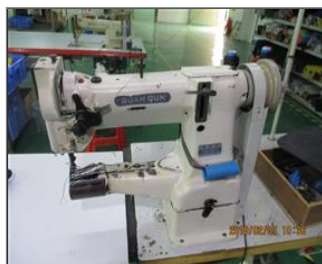
Photo of non-conformity NC-No needle plate for high speed sewing machine.JPG
